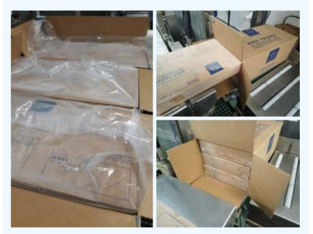
**Photos:** new packaging configuration, from top loading boxes, wrapped in plastic (left), to plastic free side loading boxes (right)
